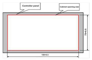
Overall size of the controller, panel: 170mm long, 85mm wide, body: 150mm long, 75mm wide, 100mm deep.
