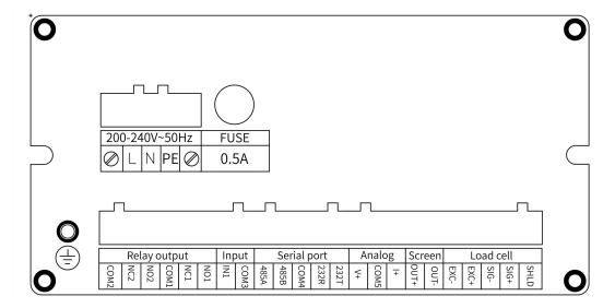
The rear panel of the DC24V power supply instrument is as follows:
